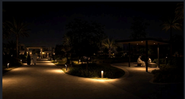
PLANTING READ BY LIGHT REFLECTED OFF THE PATH, WITH NOTHING AIMED INTO THE CANOPY.
