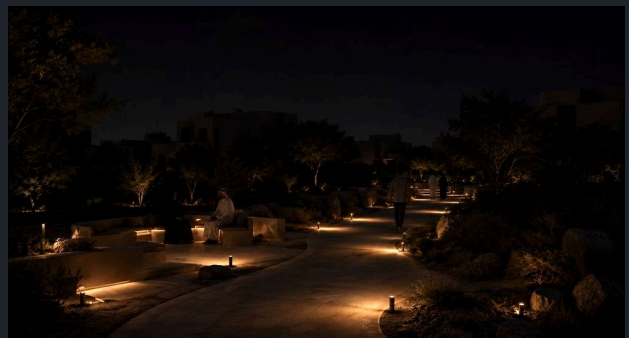
SEATING AT VERY LOW LEVEL. ENOUGH TO READ THE GROUND, NOT ENOUGH TO GLARE.
