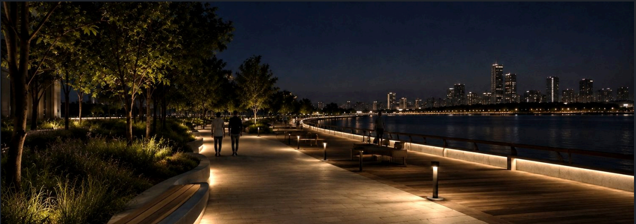
PROMENADE LIT FROM THE EDGE, SO THE LIGHT LANDS ON THE DECK AND NOTHING POINTS OUTWARD.
